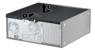
To install the access panel, reverse the removal procedure.
